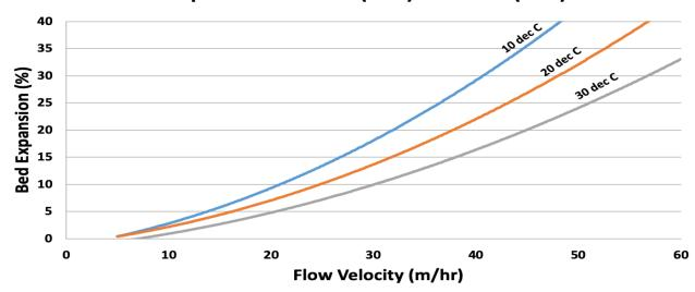
Bed Expansion is influenced by both temperature and by water density (TDS). In practise the influence of temperature is far greater than TDS. Expansion curves for seawater are therefore not significantly different from the above.
