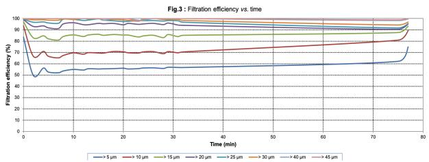
Taking 5u particle size, there was a gradual decrease in performance of AFM® which stabilised at approx 92% removal efficiency. Sand experienced a rapid drop in performance to 50% efficiency then stabilised at approx 55%.
