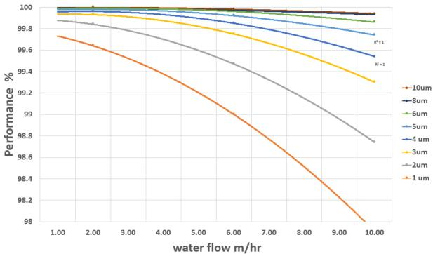
AFM® grade 0 is preferably used between water flow velocities from 1 to 10m/hr,.Filtration performance is related to filtration velocity, the slower the water flow velocity the better the performance. The above data is without any pre-coagulation of flocculation and is using ISO A4 grade silica particles.
