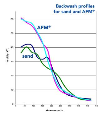
In most cases the backwash will be complete within 300 seconds, however if the bed is not fluidised, the curve will be flat and very protracted. If there is deep solids penetration into the bed, or if there is a large head space above the media, then a longer backwash will be required, not only to clean the media but also to evacuate all the water above the bed.
