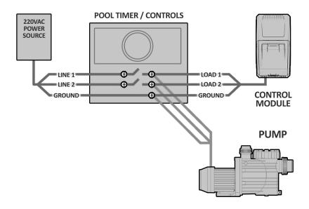
In some parts of the United States and Canada, the Control Module must be connected to a circuit protected by a Class A ground fault interrupter (GFI). Check local codes before connecting.
