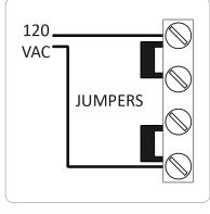
This set of terminal screws can be located inside of the Control Module, and accessed by removing the six screws from the Control Module's aluminum base. The factory voltage setting is the 240V configuration, with a jumper clip inserted between the second and third terminals. The Control Module can be made to accept 110V by reconfiguring the jumper clips as shown above right, with two jumper clips instead connecting the first & second terminals, and the third & fourth terminals.
