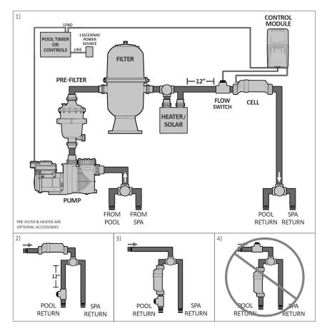
**NOTE**: The following are basic plumbing instructions for the typical installation (Configuration #1), which entails positioning the Flow Switch and Cell adjacent to each other on 2" plumbing. Your installation may vary depending on space available and your specific arrangement of equipment.
