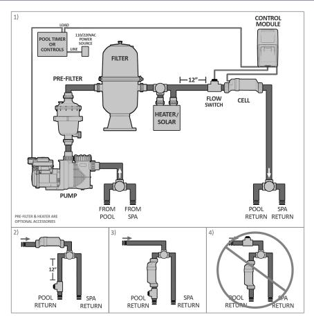
There are three main components to your Atecpool ATSGP Series system: the Control Module, the Electrolytic Cell, and the Flow Switch.
