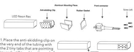
the very end of the tubing with the 2 tiny tabs that are pointing inwards still touching the end of the material and crimp in place.
