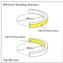
LED Neon flex is a highly durable product but must be installed in accordance to the pictures shown below, which indicate the minimum bending parameters as well as the correctly bending direction for each specific variant of model
