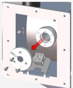
On each side, remove the lamp supports by unscrewing the 3 screws.
