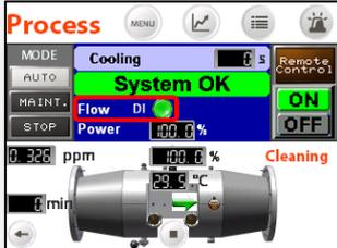
Power on the lamps by pressing the red On/off button on the screen.
