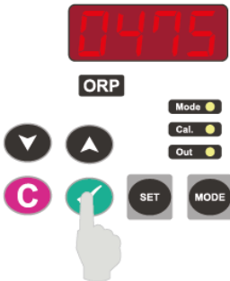
Picture 10 Single Point Calibration
