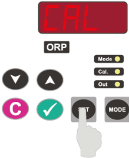
Picture 10 Single Point Calibration
