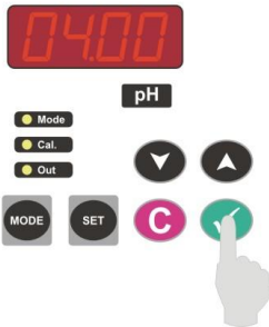
Picture 11 Double Point Calibration
